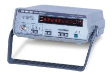
The GFC-8010H performs virtually most of the counting measurements required in laboratories, in terms of both period and frequency. 8 digits LED display with distinctive red color and overflow indicator provides fast and clear view. Easy operation with all functions neatly organized on the front panel, compact size suitable for both portable and bench-top usage, GFC-8010H serves users as a handy reference.
